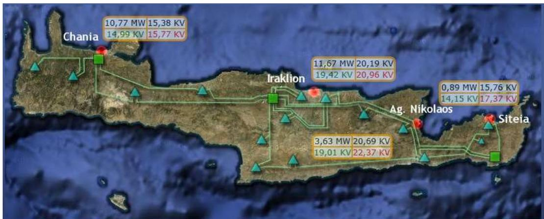
Figure 37 - Transmission Grid of Crete and optimal power flow visualization
