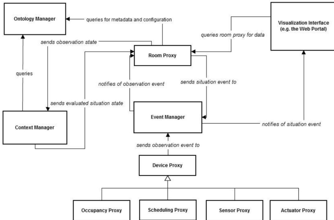
Fig. 08 – Interaction between components in the SEEMPubS system.
