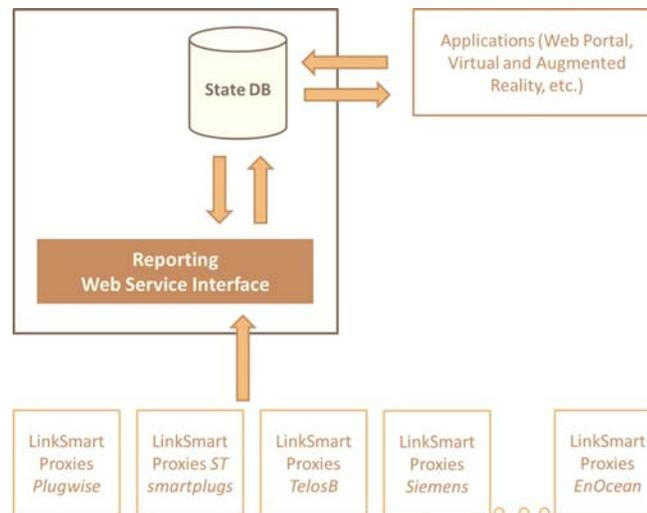
Fig. 02 – The SEEMPUBS State DB Architecture.
