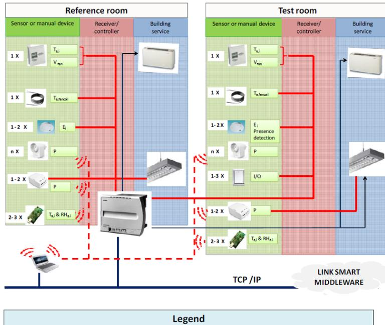
Fig. 05 – Example of wired & wireless architecture designed for the Main Campus.
