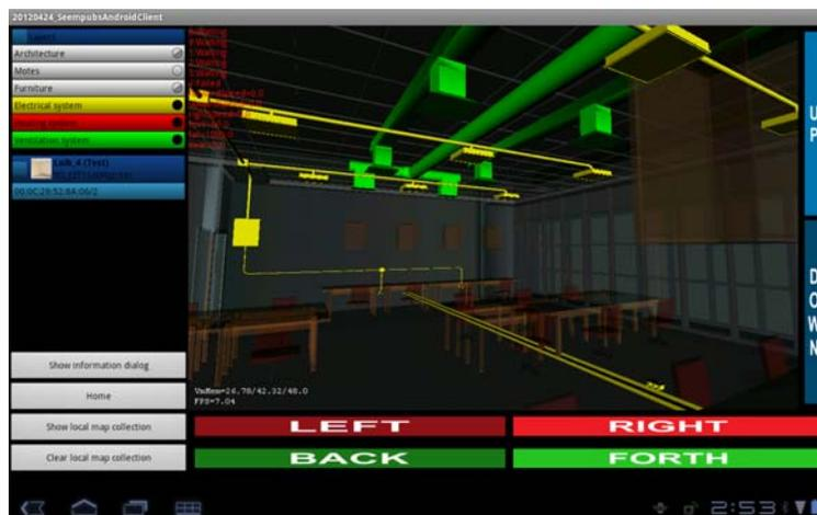
*Fig. 13 – Visualization of architectural and system using a BIM model visualized into a tablet.*
