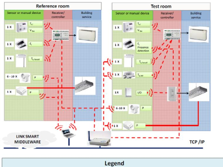
Fig. 06 – Wireless architecture designed for the DITER Offices in the Valentino Castle.
