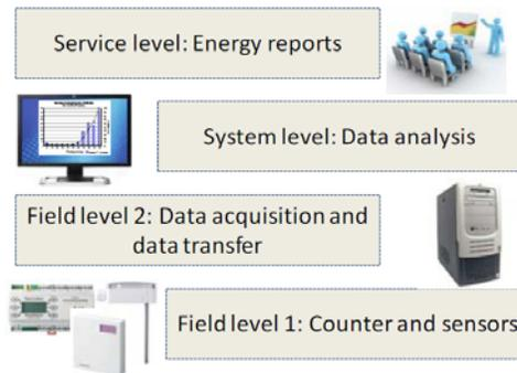
Fig. 07 – Four levels for ongoing/continuous control and monitoring system.
