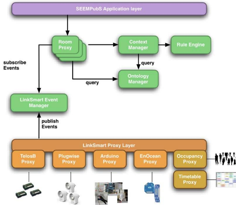
Fig. 10 – SEEMPubS software architecture.
