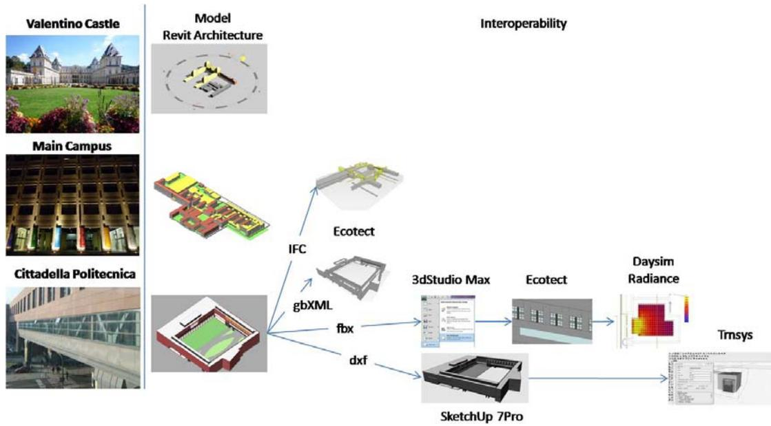
Fig. 11 – Conceptual map of data exchange between interoperable software.
