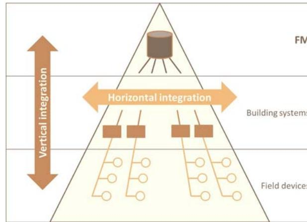
Fig. 01 – Horizontal and vertical integration in the SEEMPubS project.
