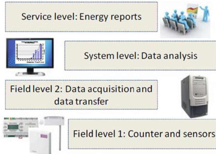
**Figure 1: Four levels for on-going/continuous control and monitoring system [D5.1]**
