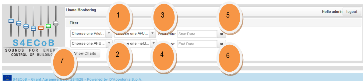
Figure 9 - Linate BMS monitoring web page: analysis selection
