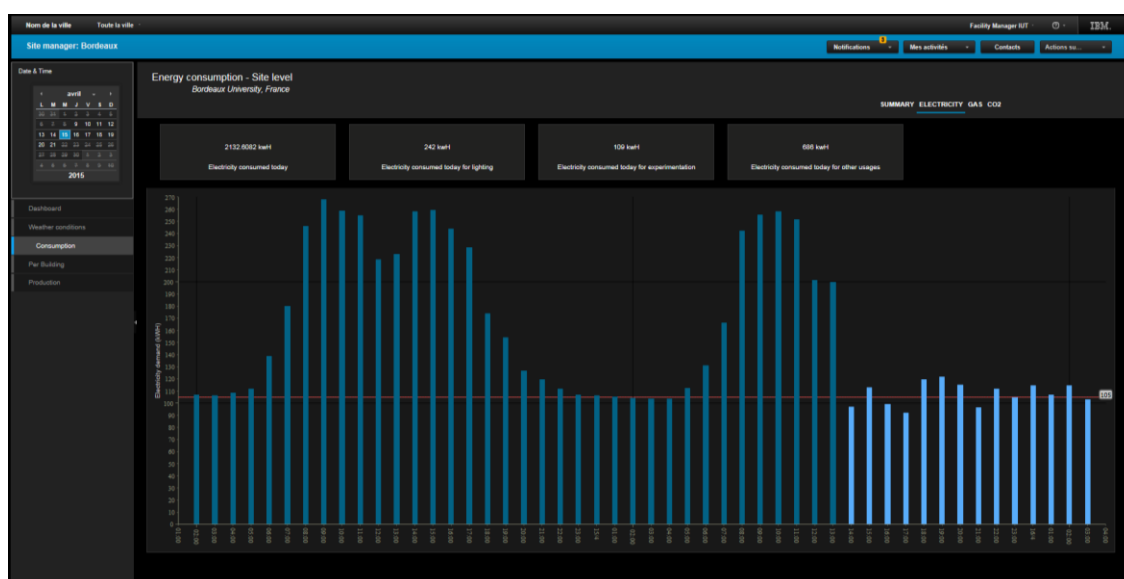
Figure 22: Hourly electricity consumptions versus time for the whole IUT site – EPNSP interface
