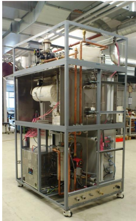
Figure 2-1: The SOFC based \mu -CHP unit
