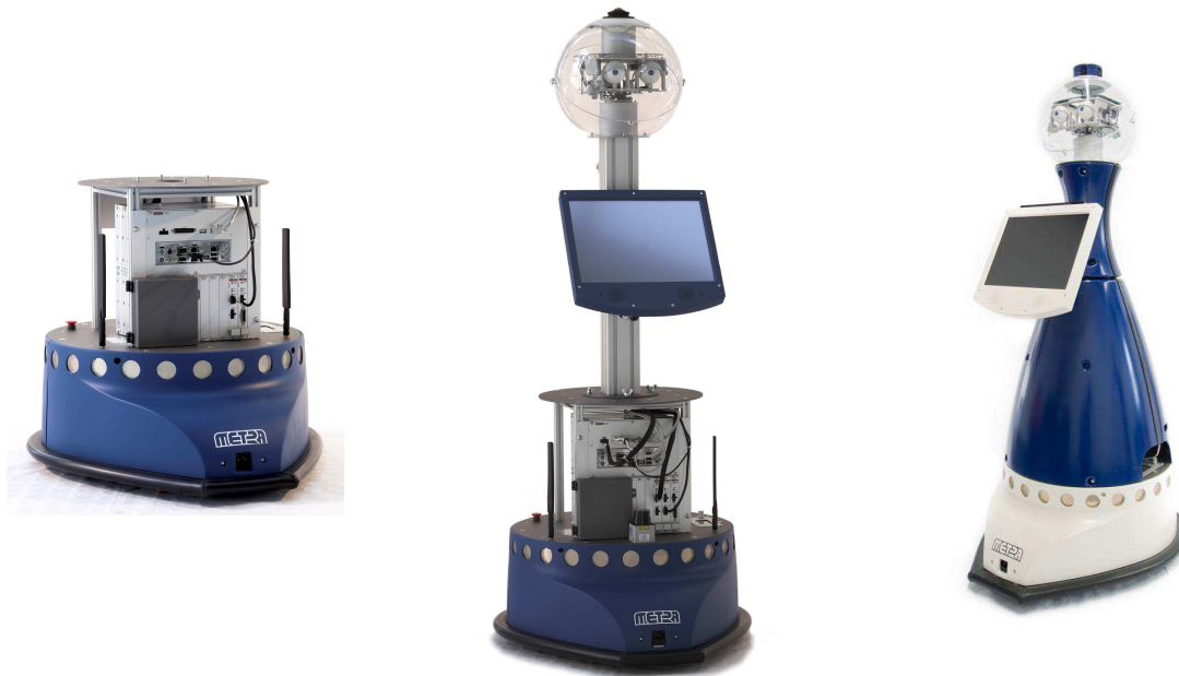
Figure 10. The MetraLabs SCITOS G5 mobile robot platform base module (left), with additional human-machine interface module (middle) and casing closed (right).
