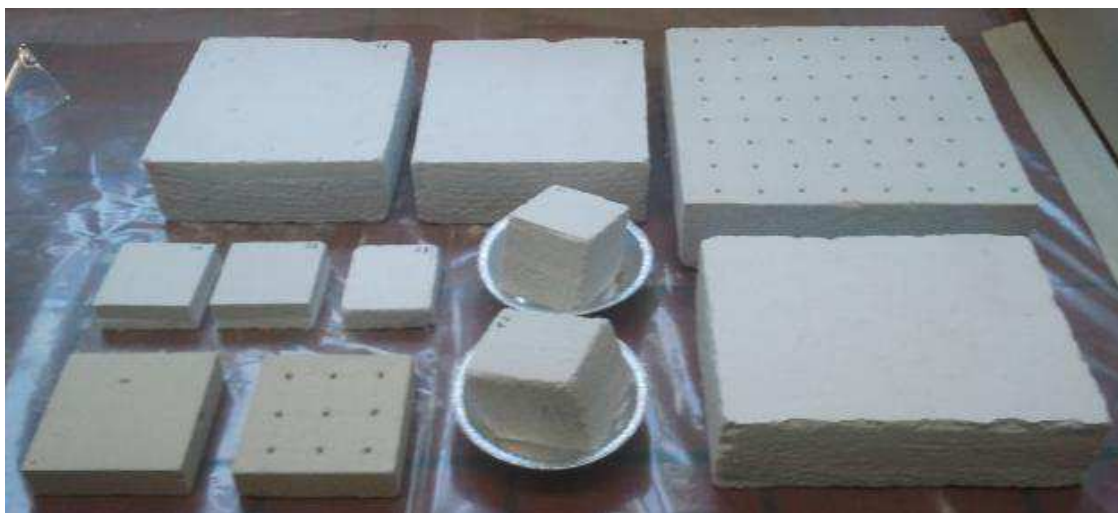
Fig. 21: Perlite specimens, with and without hydrophobic agent, ready for testing.
