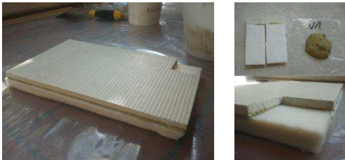
Fig. 25: Sample of sandwich panel after gluing aerogel mat to the Recycled glass board.
