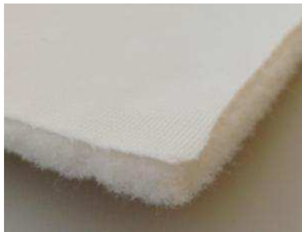
Fig. 14: Example of Aerogel containing non-woven PES mat coupled with a white tri-laminate Polyester-finishing textile.
