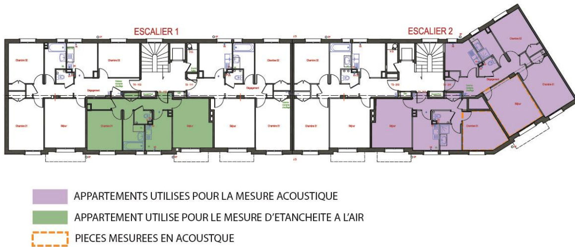
Figure 64: Location of dwellings in which the acoustic tests after refurbishment were performed (purple zone)
